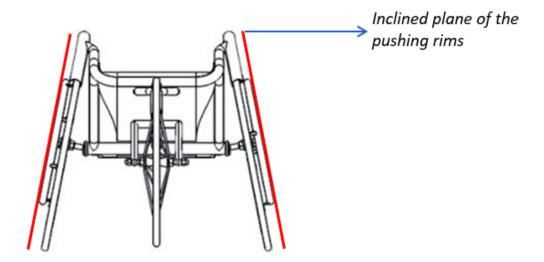
Figure 4 – Inclined plane of the pushing rims
