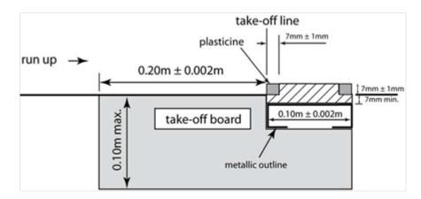
Figure 9 – Take-off board and plasticine indicator board
